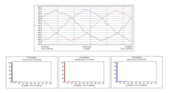
Ithd after filtration ranges at a very low 5.11% to 6.38%. Of note is the IEEE519-2022 compliance criteria would be 8.0% based on the SC ratio of the application. It should be noted that the testing was being conducted at a load profile of 52% of full load current, which would indicate the Ithd measured would be even lower at higher load profiles. The current harmonic witnessed significantly exceeded the IEEE requirements. Note the comparative of the power profiles below:
