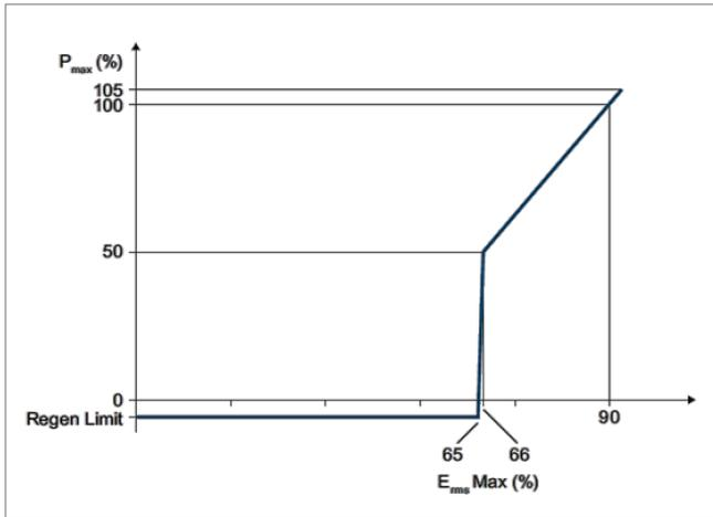
Figure 8. Drive Power (Pmax) as a Function of Input Voltage Magnitude (Erms)
