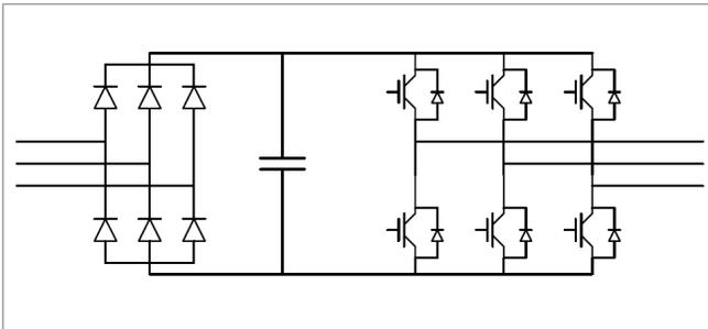
Figure 6. 6 Pulse 2 Level Low Voltage Inverter
