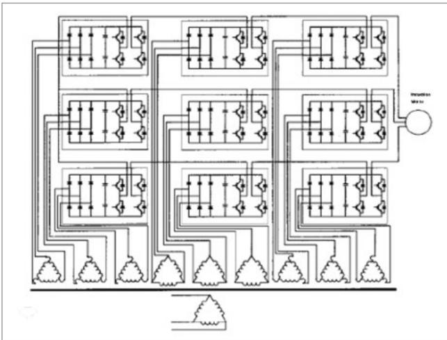
Figure 7. Multilevel H-Bridge Medium Voltage Inverter
