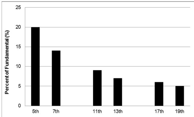
Figure 9. Theoretical harmonic magnitude (per unit) quasi square wave
