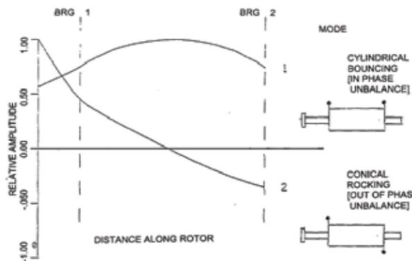
Figure 9 Rotor Mode Shape at Critical Speed
