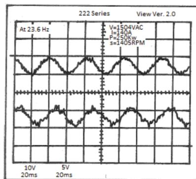
Figure 6 Voltage and Current Waveform (23.6 Hz)
