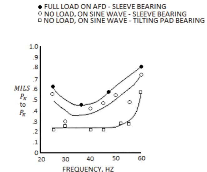
Figure 15 Measured Shaft Vibration
