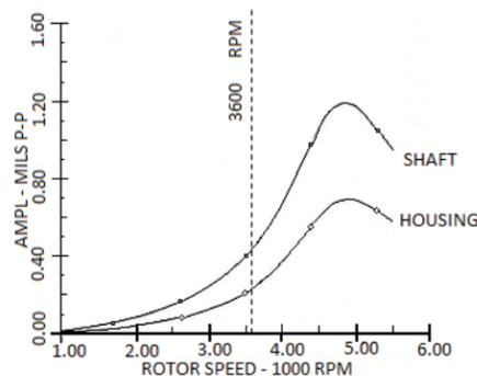
Figure 12 Calculated Unbalance Response - Tilting Pad Bearings
