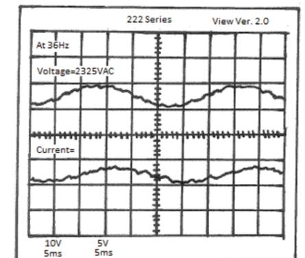
Figure 5 Voltage and Current Waveform (36 Hz)
