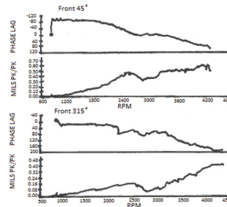
Figure 13 Coastdown Test - Shaft Relative Vibration Runout Compensated for in Phase Unbalance
