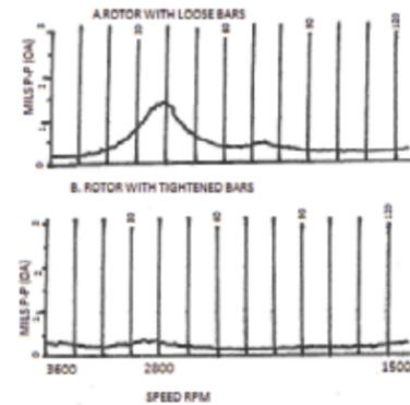
Figure 16 Rotor Coastdown in Balance Machine before and after Tightening Bars
