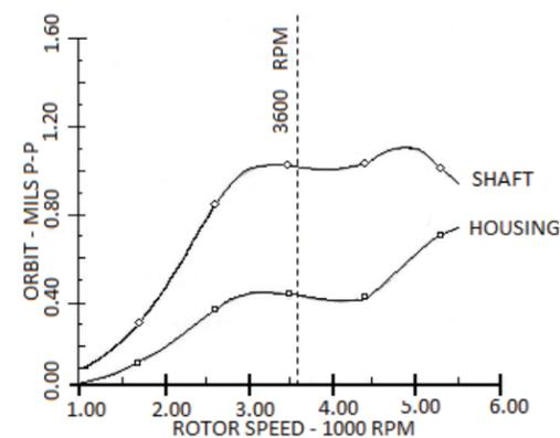
Figure 11 Calculated Unbalance Response Orbital Plot - Sleeve Bearings
