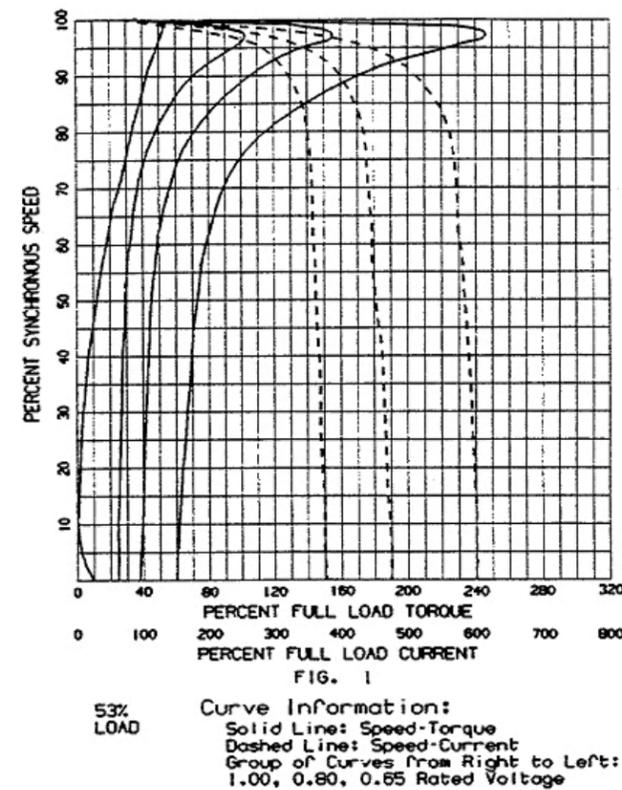
Figure 1 Speed torque curves of all applications
