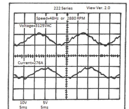
Figure 4 Voltage and Current Waveform (48 Hz)
