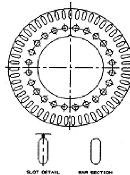
Figure 2 Rotor lamination/ axial vent holes
