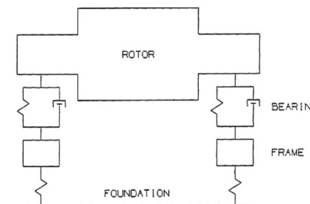
Figure 8 Schematic of Rotor Bearing System
