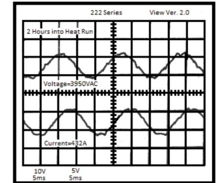
Figure 3 Voltage and Current Waveform (60 Hz)
