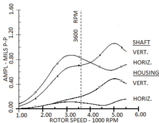
Figure 10 Calculated Unbalance Response - Sleeve Bearings
